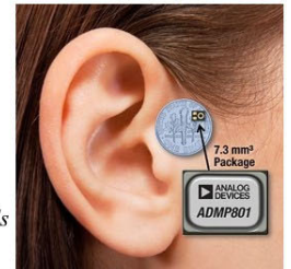
MEMS microphone (Analog Devices)
