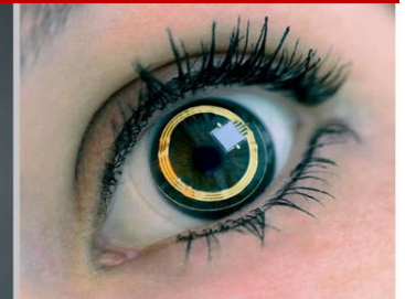
MEMS implantable pressure sensor (Sensimed)
