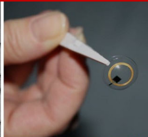
MEMS implantable pressure sensor (Sensimed)
