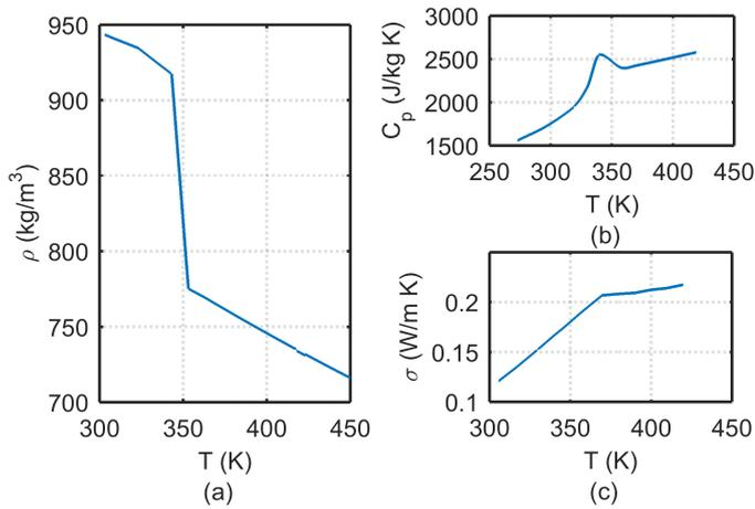
Fig. 3. Thermophysical properties of Hexatriacontane used in multiphysics simulation (a) density (b) heat capacity (c) thermal conductivity.
