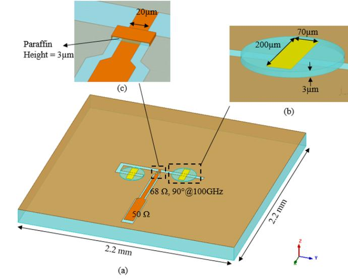
Fig. 1. (a) 3D view of the reconfigurable slot antenna with paraffin PCM capacitors, (b) detailed view of the paraffin PCM capacitor, and (c) detailed view of the bridge.
