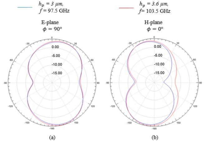
Fig. 8. Radiation pattern of the proposed antenna for paraffin thickness of 3  $\mu\text{m}$  and 3.6  $\mu\text{m}$ . Antenna has a maximum gain of 3.78 dBi.
