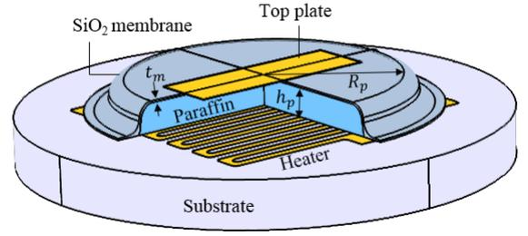
Fig. 2. 3D schematic of the electro-thermo-mechanical paraffin actuator with micro-heater, paraffin cavity and SiO<sub>2</sub> membrane.
