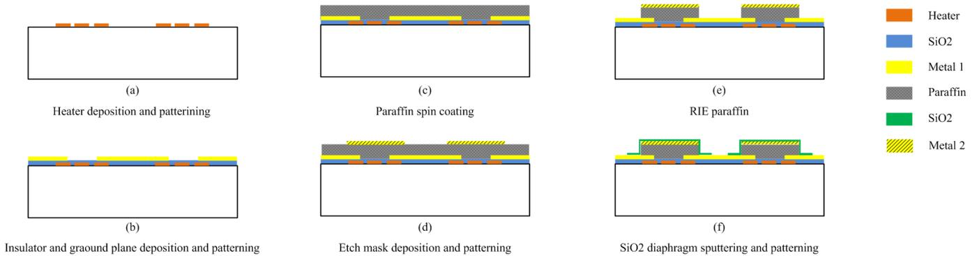
Fig. 6. Simplified fabrication process flow of the reconfigurable slot antenna.
