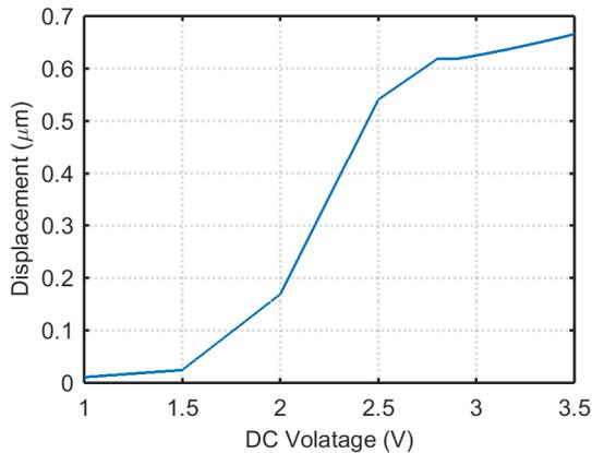
Fig. 4. Displacement of the actuator membrane (at the center) as a function of the bias voltage.
