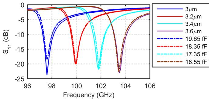
Fig. 7. Simulated  $S_{11}$  of the reconfigurable slot antenna for various paraffin thickness.
