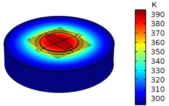
Fig. 5. Temperature distribution (units in K) of the actuator at DC bias voltage of 3.5 V.
