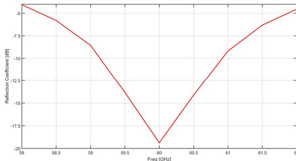
Fig. 3: Simulation results showing reflection coefficient ( $S_{11}$ ) as a function of frequency. Minimum  $S_{11}$  is  $-19$  dB and bandwidth is approx. 1.7 GHz.
