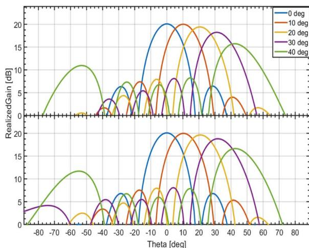
Fig. 4: Simulation results for the antenna pattern showing realized gain as a function of scanning angle for  $E$ -plane (top) and  $H$ -plane (bottom).
