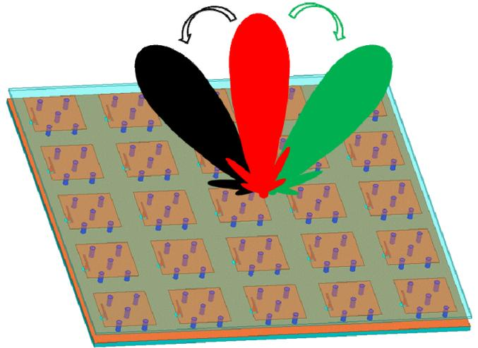
Fig. 2: 3D schematic of high-efficiency phased array with 25 elements. Each patch is suspended on 5 posts and fed by capacitive pin.
