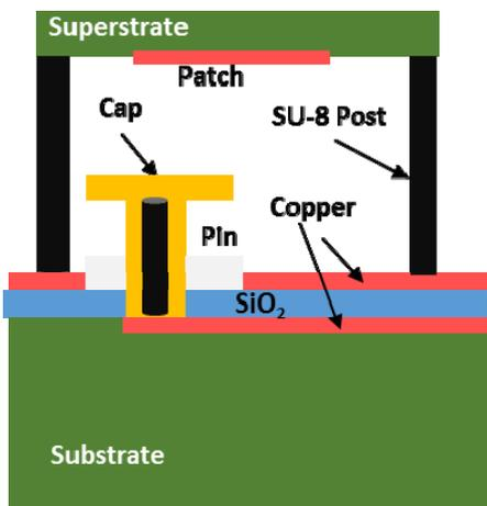
Fig. 1: Schematic cross section of the proposed pin-fed suspended patch array.
